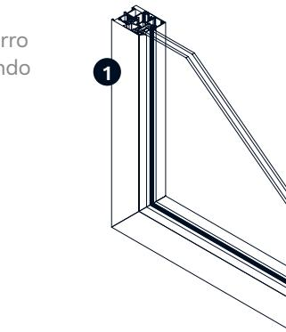
① Aluminum profile with thermal break
